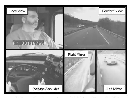
Figure 3. Photo. Five Camera Images Multiplexed Into a Single Image
