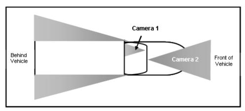
Figure 1. Diagram. Camera Directions and Approximate Fields of View
